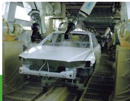
Automobile body coating line Photo: Mazda's 3 wet-on coating system clear coating process
