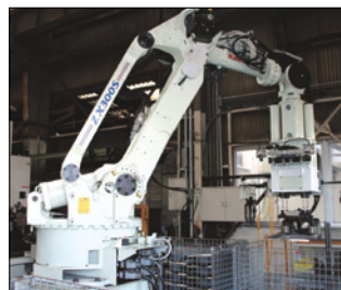
Releasing and loading/unloading of large-sized workpieces using vision system
