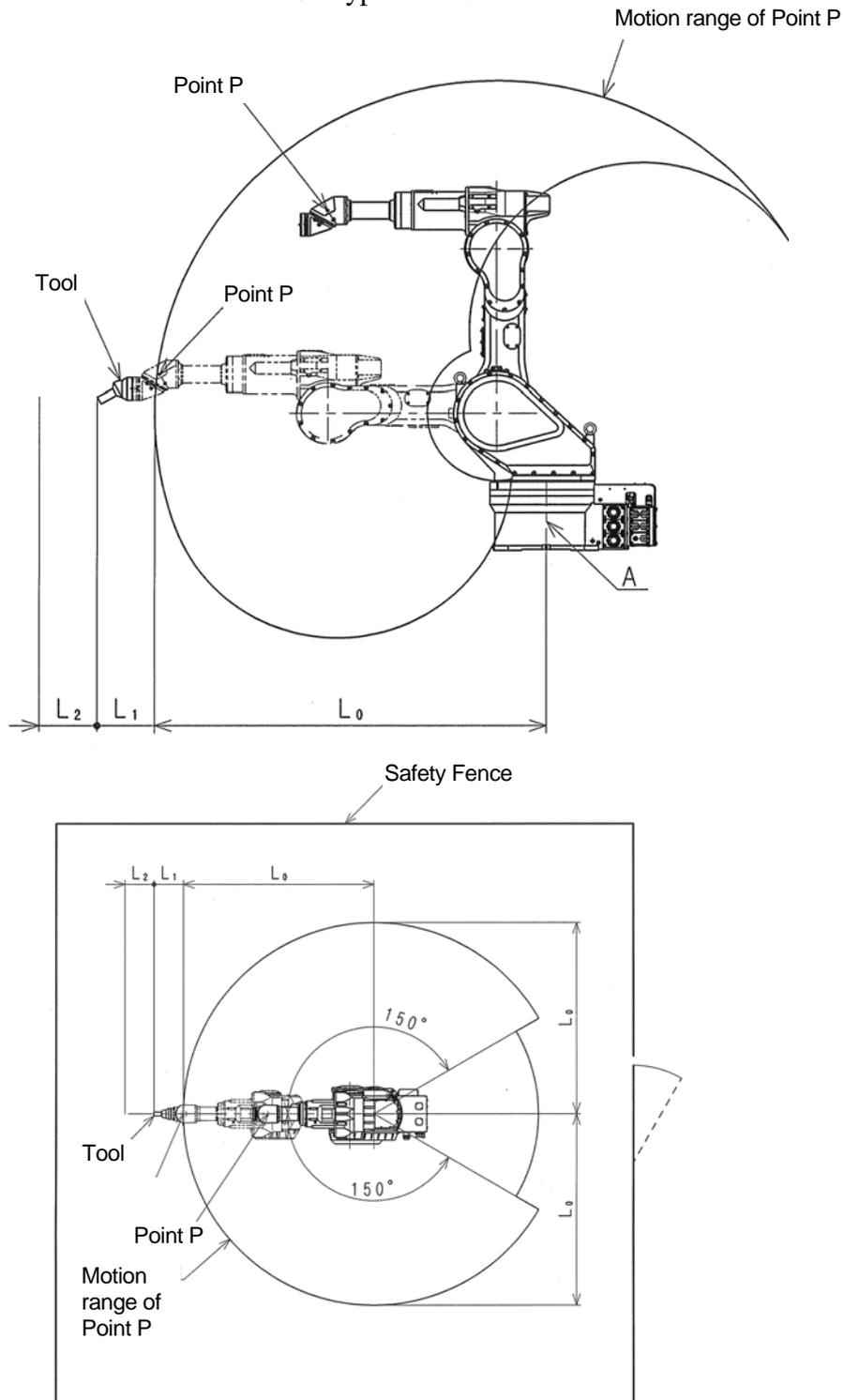
The motion range of robot arm is represented by Point P in the figure above. Accordingly, the dimensions of safety should be calculated as follows: Determine sum of  $L_0$ ,  $L_1$  and  $L_2$  as minimum dimension. That is: dimension from the center of arm (Point A shown in the figure above) to the center of wrist ( $=L_0$ ) + dimension from the center of wrist to the edge of tool ( $=L_1$ ) + dimension of allowance ( $=L_2$ ).
