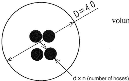
$$\text{volume ratio} = \frac{\underbrace{d^2}_{\text{Area of hose(s)}} \pi n}{\underbrace{D^2}_{\text{Area of wrist hollow}}} \pi \times 100 [\%]$$
