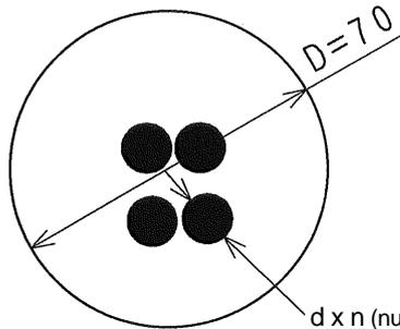
$$\text{volume ratio} = \frac{\underbrace{d^2}_{\text{Area of hose(s)}} \pi n}{\underbrace{D^2}_{\text{Area of wrist hollow}}} \pi \times 100 [\%]$$
