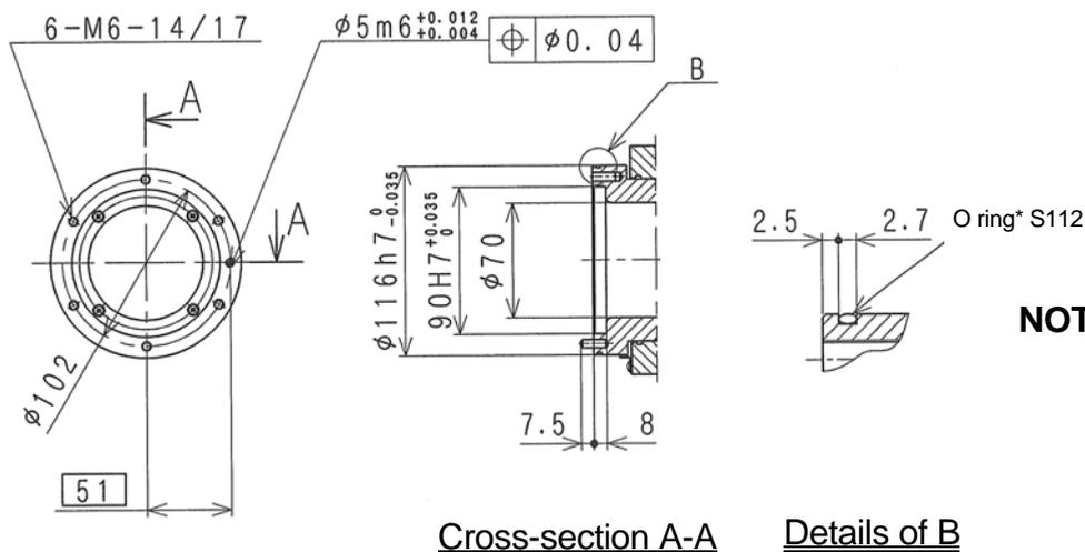
**NOTE\*** When removing or replacing tools, replace the O-ring, too.
