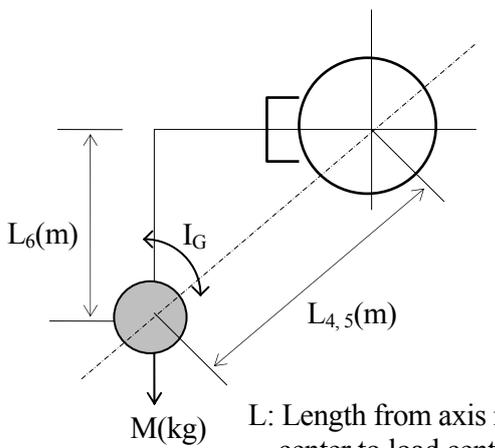
$L$ : Length from axis rotation center to load center of gravity (Unit: m) (See the figure.)
