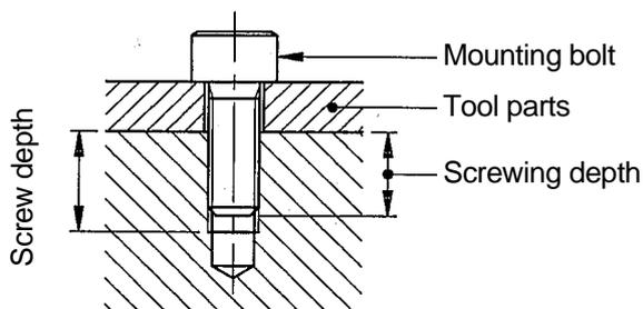
Select mounting bolts with proper length to secure the specified screwing depth according to the screw depth of tool mounting flange. Use high tension mounting bolts and tighten them to the specified torque.
