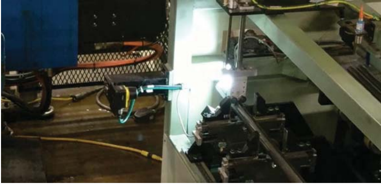
The Laser Seam Finder uses a Cognex camera to locate a notch in the front of the round pipes, which signifies the pipe's weld seam is in the proper position.
