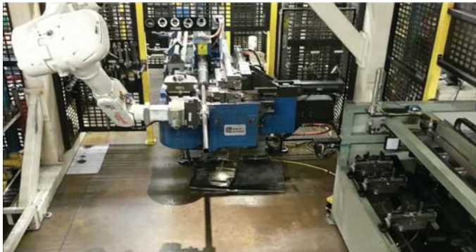
Inside KMM's Bender Bot 1 cell, which uses one RS050N robot to load and unload a tube bending machine.
