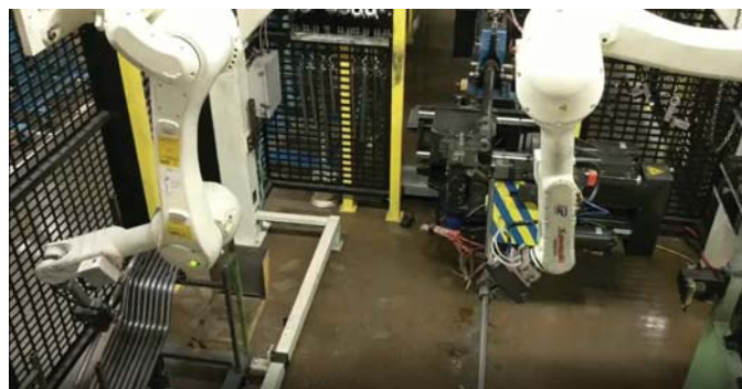
KMM's Bender Bot 2 cell uses two Kawasaki RS020N robots to load and unload smaller pipes with the goal of increasing throughput.
