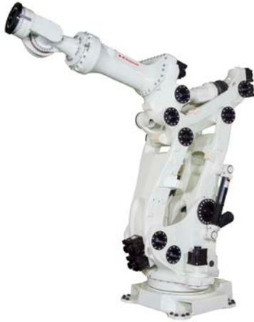
Kawasaki Robot announced that it will release the MG10HL, a highly rigid, ultra-high payload robot on December 2, 2015. It boasts a maximum payload capacity of one ton, the largest among Kawasaki robots.
