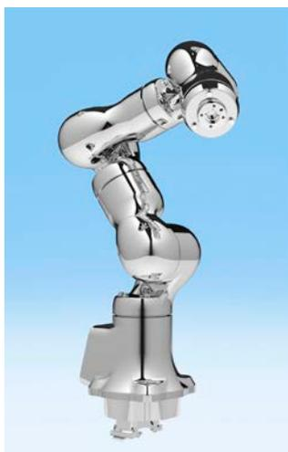
A tooling cable can be placed inside of the arm each robot and run all the way to the apical flange, helping to minimize interference with peripheral equipment. Both models can be installed in confined spaces, or mounted on top of peripheral equipment.
