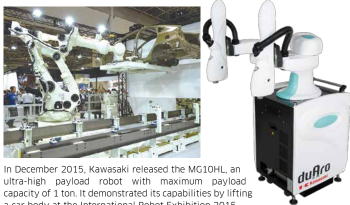
duAro, a dual-arm SCARA robot suitable for multi-product and small-lot productions collaborating with people safely and securely.
