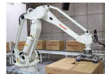
In October 1999, 7 models of the large general-purpose Z series robots, with a class-leading working envelope, were launched. Photo is the ZD250 performing the palletizing work exhibited at the International Robot Exhibition 2013.
