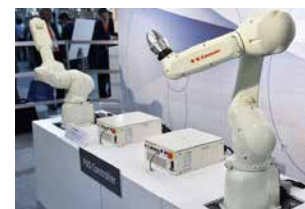
In December 2016, the industry’s smallest and lightest small robot controller, the F controller, was launched. At the International Robot Exhibition 2017, the small general-purpose RS007N and RS007L robots demonstrated high speed operations using the F controllers.
