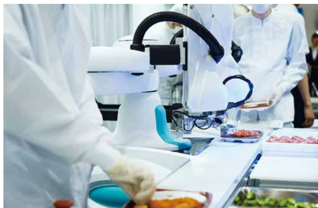
duAro, a dual-arm SCARA robot suitable for multi-product and small-lot productions collaborating with people safely and securely.
