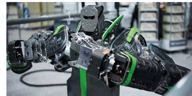
The humanoid robot announced at the International Robot Exhibition 2017 is an endoskeleton-type measuring 175cm tall and weighs 80kg. In a demonstration, it lifted up dumbbells as heavy as the robot itself and showed its ability to get up after falling.
