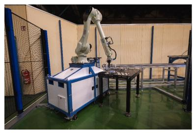
+For additional flexibility, another industrial robot is used on a mobile shuttle system. This robot picks up the empty perforated plates, transports them to the Kawasaki Robotics RS010L and transports the loaded plate to the final assembly at the manual workstation.
