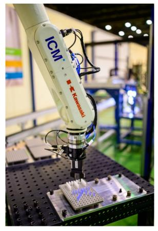
The Kawasaki Robotics RS010L mounts the desired pin configuration on a provided plate and handles it between the conveyor belt and the mobile unit.
